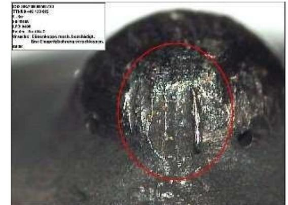
Foreign Particle In Combustion Chamber
