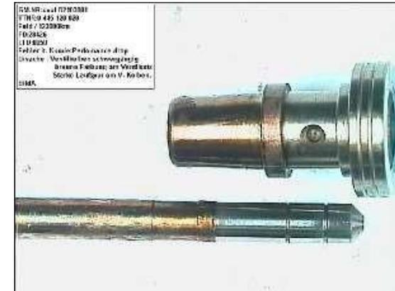
Sluggish Valve Piston Or Nozzle Needle
