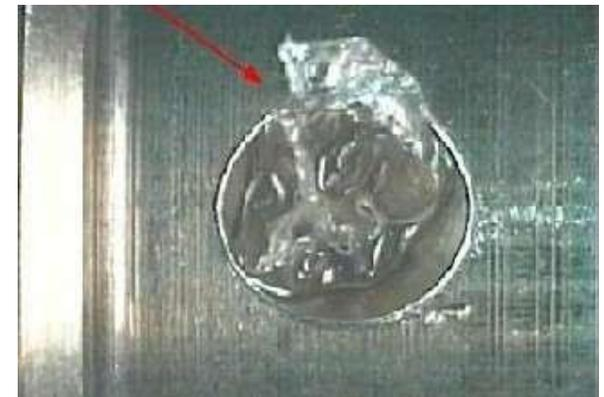
Sluggish Valve Piston Or Nozzle Needle
