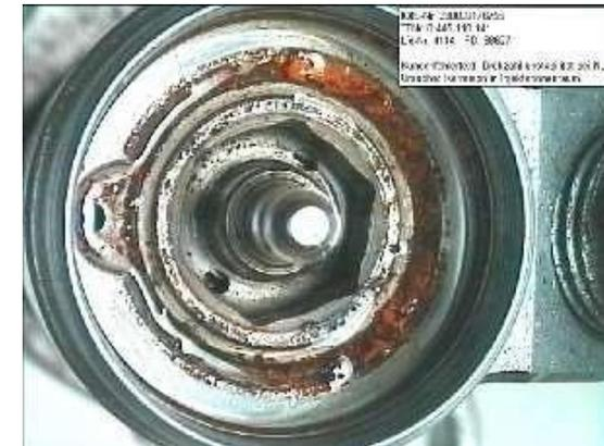
Sluggish Valve Piston Or Nozzle Needle
