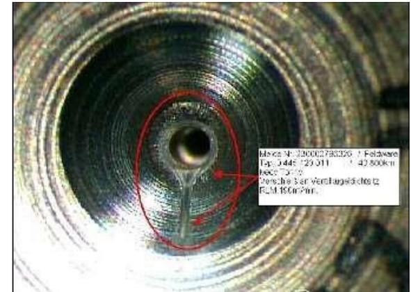
Beyond Repair Damage To Valve Seat
