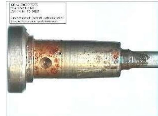
Sluggish Valve Piston Or Nozzle Needle
